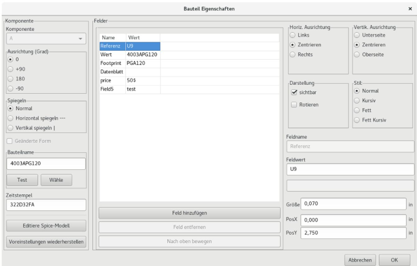
The Symbol Properties window displays all the fields of a symbol in a table. New fields can be added, and existing fields can be deleted, edited, reordered, moved, or resized.
