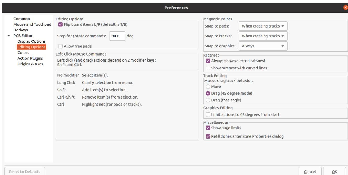
**Flip board items L/R:** Controls the direction board items will be flipped when moving them between the top and bottom layers. When checked, items are flipped Left-to-Right (about the Vertical axis); when
