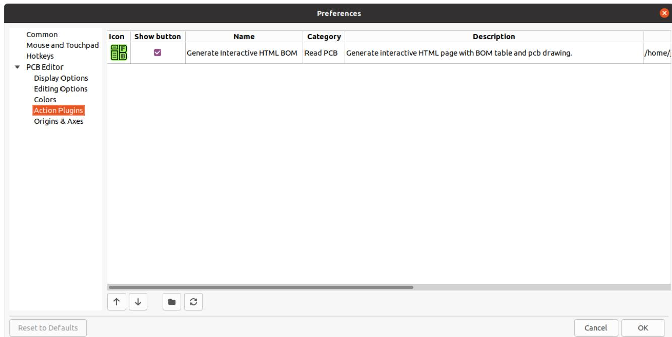
The KiCad PCB editor supports plugins written in Python that can perform actions on the board being edited. These plugins can be installed using the built-in Plugin and Content Manager (see the KiCad chapter for details) or by placing the plugin files inside the user plugins directory. See the Scripting section below for details.
