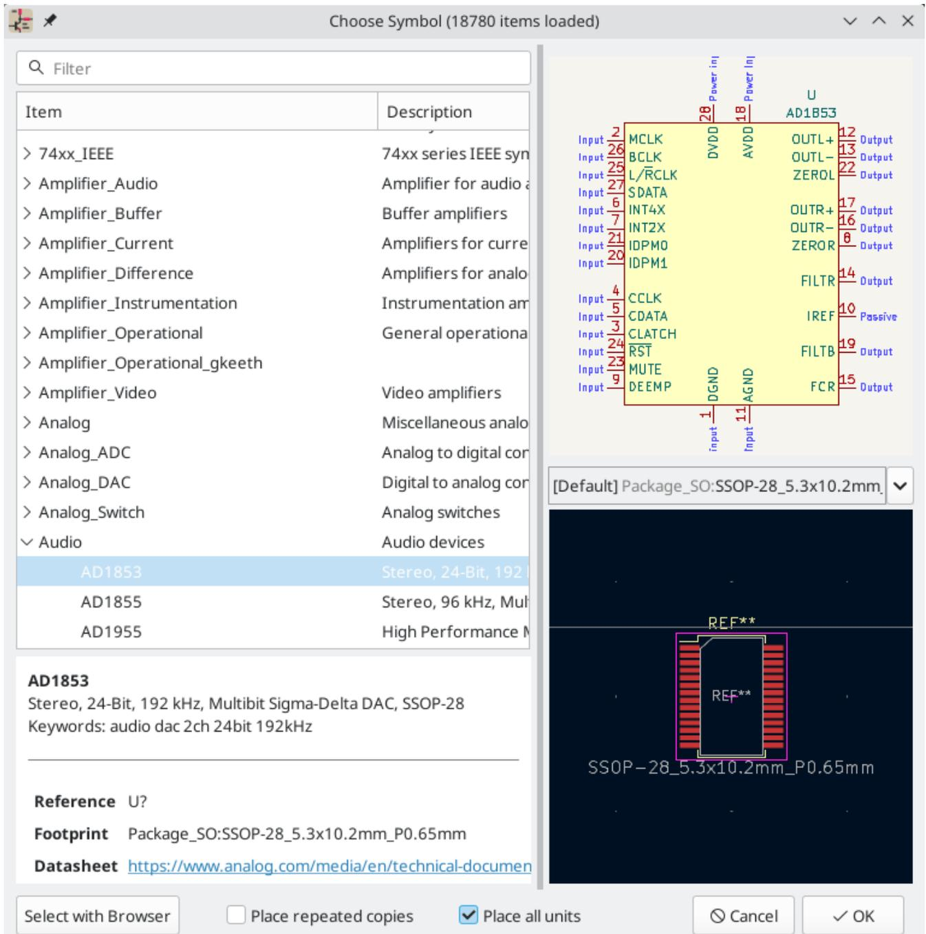
Symbols can have footprint filters that specify which footprints are appropriate to use with that symbol. If footprint filters are defined for the selected symbol, all footprints that match the footprint filters will appear as options in the footprint dropdown. The selected footprint will be displayed in the preview canvas and will be assigned to the symbol when the symbol is added to the schematic.
