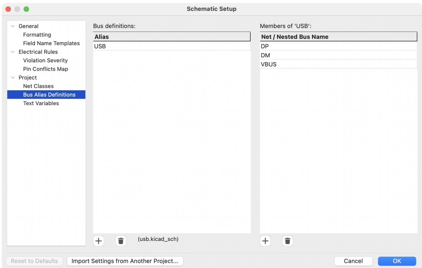
An alias may be named any valid signal name. Using the dialog, you can add signals or vector buses to the alias. As a shortcut, you can type or paste in a list of signals and/or buses separated by spaces, and they will all be added to the alias definition. In this example, we define an alias called `USB` with members `DP`, `DM`, and `VBUS`.
