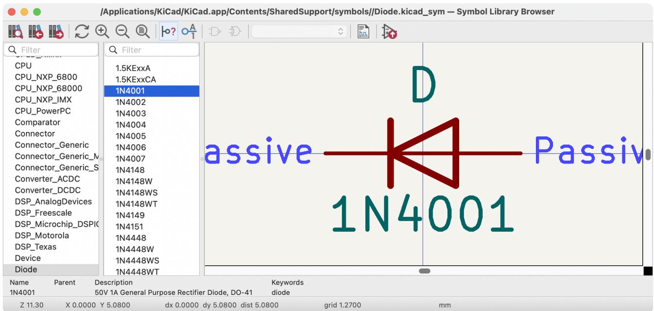
Double clicking the name of a symbol or using the
