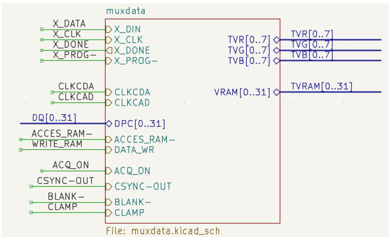
For every hierarchical label in the subsheet, import the corresponding hierarchical pin into the sheet symbol by clicking the
