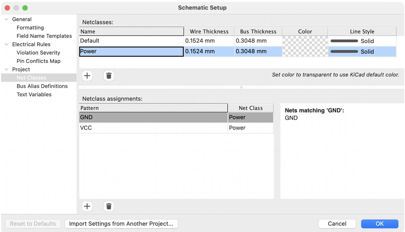
The top pane lists the netclasses that exist in the design. The `Default` netclass always exists, and you can add additional netclasses with the **+** button or remove the selected netclass with the **🗑** button.
