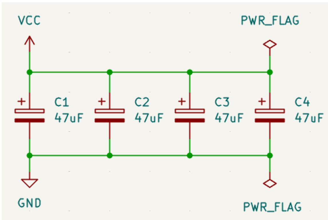
In the KiCad standard library, power symbols are found in the `power` library, but power symbols can be created in any library. To create a custom power symbol, make a new symbol with a power input pin that is set to be invisible. Name the pin according to the desired power net. In addition, set the "Define as power symbol" symbol property. As described in the [hidden power pins section](#), invisible power input pins make
