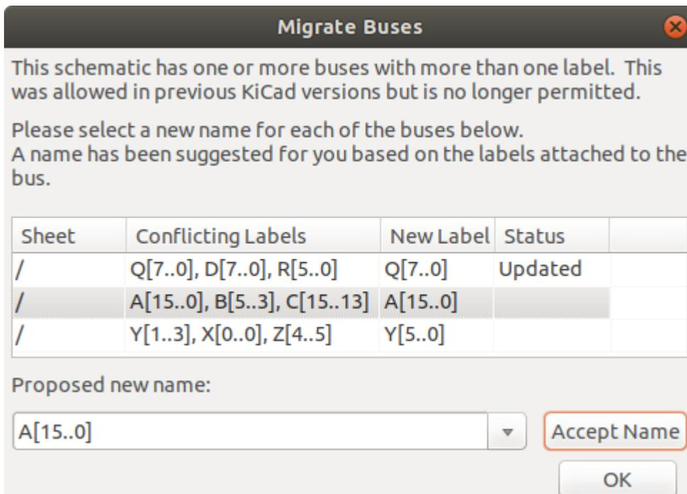
For each set of bus wires that has more than one label, you must choose the label to keep. The drop-down name box lets you choose between the labels that exist in the design, or you can choose a different name by manually entering it into the new name field.
