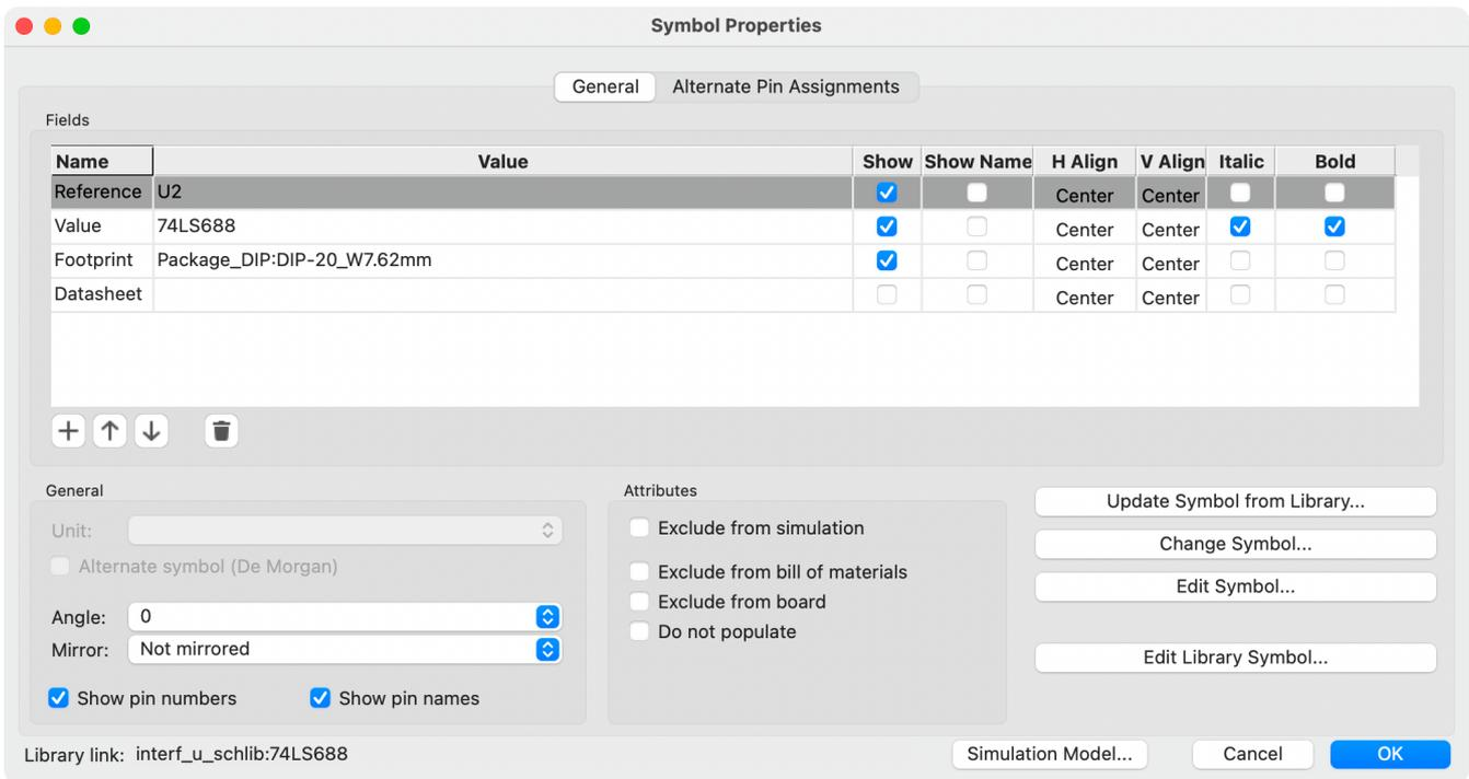
The Symbol Properties window displays all the fields of a symbol in a table. New fields can be added, and existing fields can be deleted, edited, reordered, moved, or resized.
