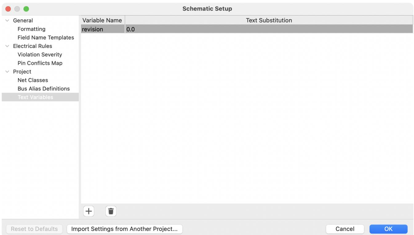
Text replacement variables can be created in the Text Variables section. These variables allow you to substitute the variable name for any text string. This substitution happens anywhere the variable name is used inside the variable replacement syntax of `${VARIABLENAME}`.
