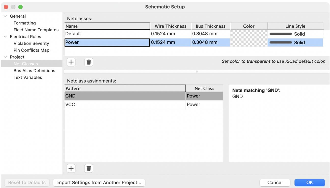
The **Net Classes** panel allows you to manage netclasses for the project and assign nets to netclasses with patterns. Managing netclasses in this panel is equivalent to managing them in the [Board Setup dialog](#). Nets can also be assigned to netclasses in the schematic using graphical assignments with [net class directives](#) or [net labels](#).
