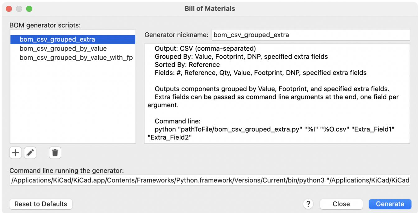
The BOM tool uses an external script to process the design information into the desired output format. Several BOM generator scripts are included with KiCad, and users can also create their own. BOM generator scripts generally use Python or XSLT, but other tools can be used as long as you can specify a [command line](#) for KiCad to execute when running the generator.
