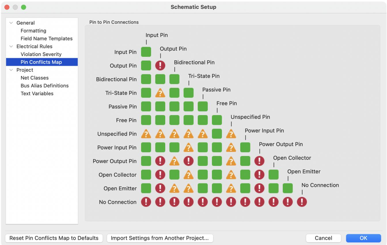
Rules can be changed by clicking on the desired square of the matrix, causing it to cycle through the choices: allowed, warning, error.
