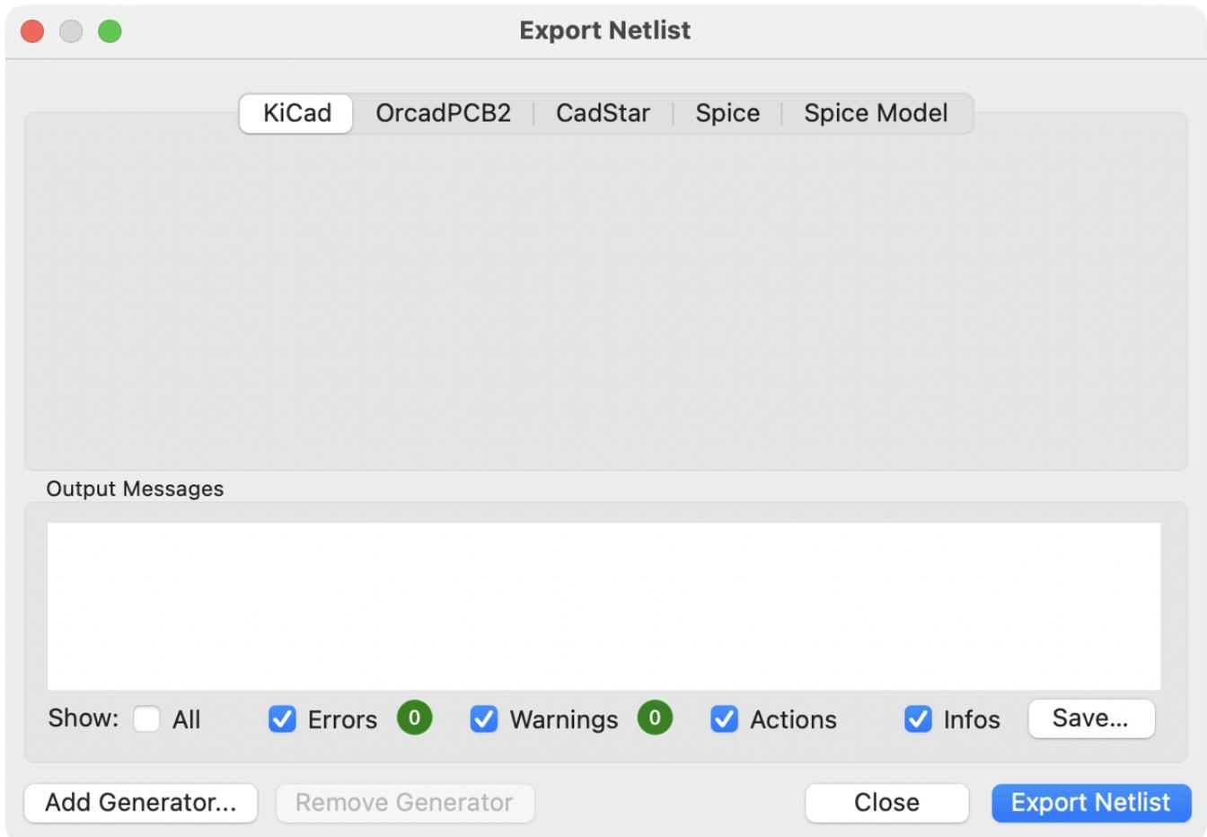
KiCad supports exporting netlists in several formats: KiCad, OrcadPCB2, CADSTAR, Spice, and Spice Model. Each format can be selected by selecting the corresponding tab at the top of the window. Some netlist formats have additional options.
