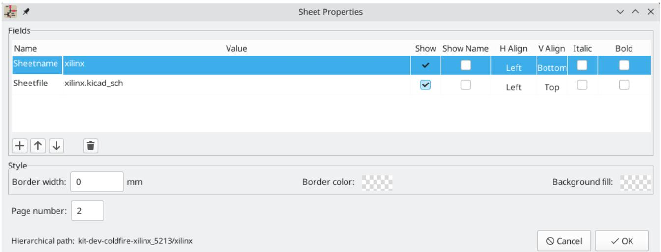
The **sheet name** must be unique, as it is used in the full net name for any nets in the subsheet. For example, a net with the local label `net1` in the sheet `sheet1` would have a full net name of `/sheet1/net1`. The sheet name is also used to refer to the sheet in various places in the GUI, including the [title block](#) and the [hierarchy navigator](#).
