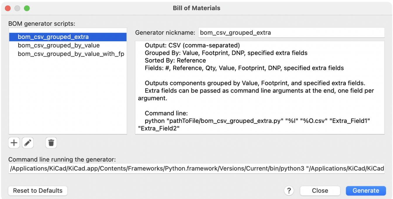
Additional scripts can be added to the list of BOM generator scripts by clicking the **+** button. Scripts can be removed by clicking the **🗑** button. The **📝** button opens the selected script in a text editor.
