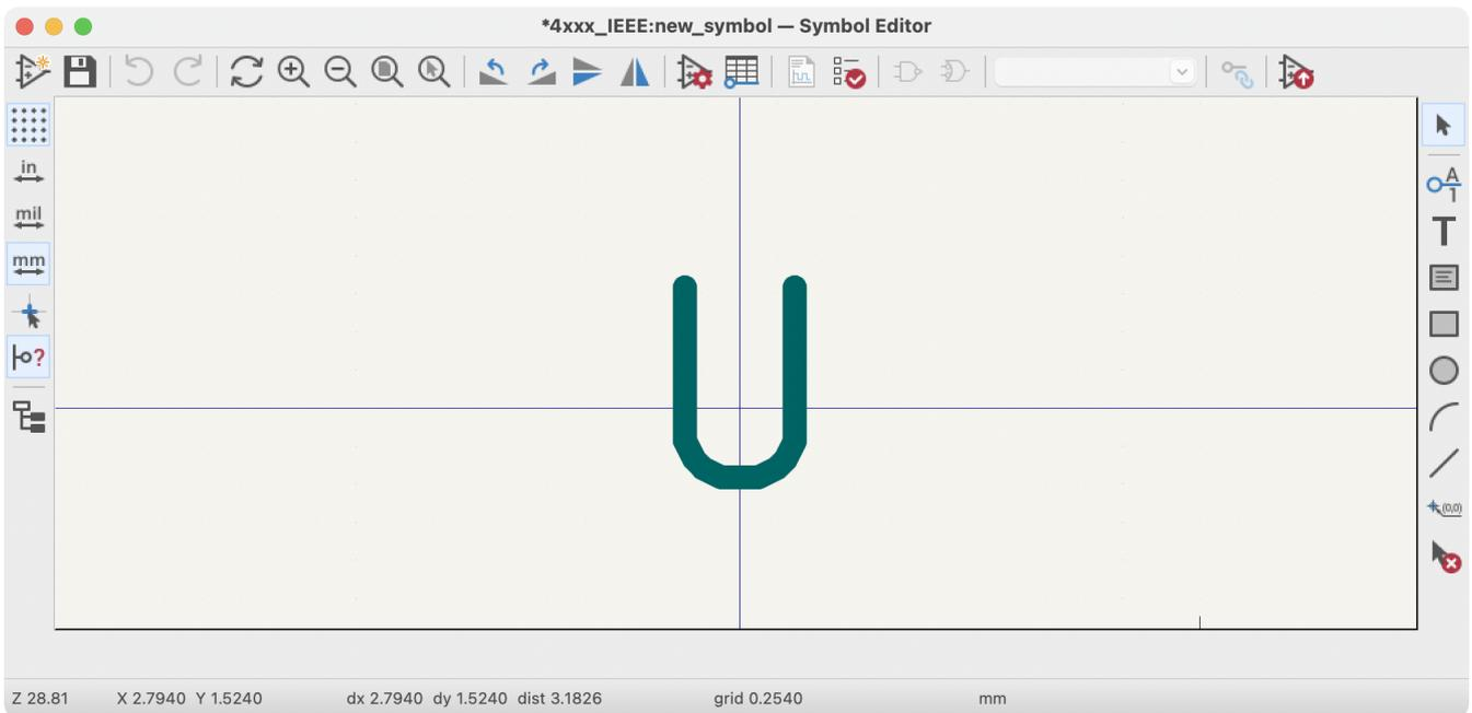
The blue cross in the center is the symbol anchor, which specifies the symbol origin i.e. the coordinates (0, 0). The anchor can be repositioned by selecting the
