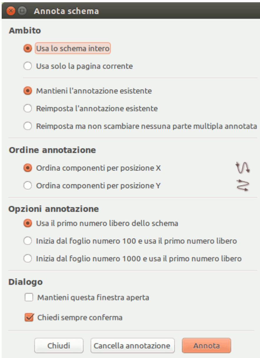
The tool provides several options to control how symbols are annotated.
