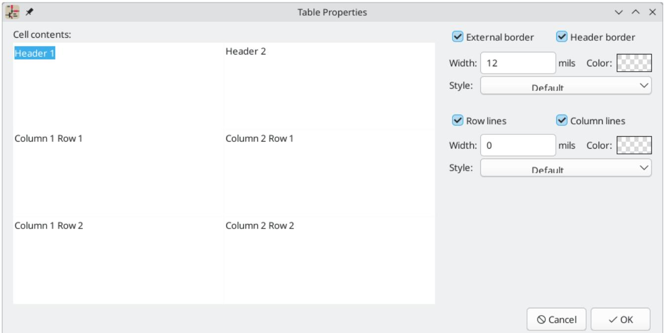
This dialog lets you edit the properties of the entire table, including the text in each cell and the separators between cells. To change the formatting of text in a cell, edit the properties of individual cells, instead of the properties for the entire table.
