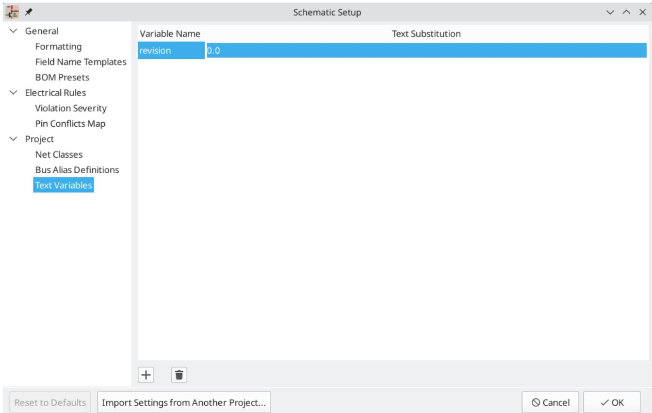
Text replacement variables can be created in the Text Variables section. These variables allow you to substitute the variable name for any text string. This substitution happens anywhere the variable name is used inside the variable replacement syntax of `${VARIABLENAME}`.
