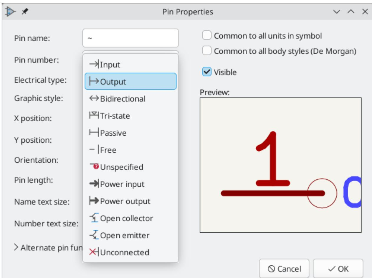
Choosing the correct electrical type is important for the schematic ERC tool. ERC will check that pins are connected appropriately, for example ensuring that input pins are driven and power inputs receive power from an appropriate source.
