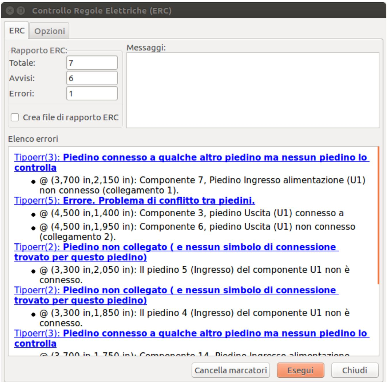
Any warnings or errors are reported in the **Violations** tab, and markers for each violation are placed in the schematic so that they point to the relevant part of the schematic. Warnings are indicated by yellow arrows, and errors have red arrows. Excluded violations are shown as green arrows. A list of the ignored tests are shown in the **Ignored Tests** tab. A report file in plain text format can be created after running DRC using the **Save...** button.
