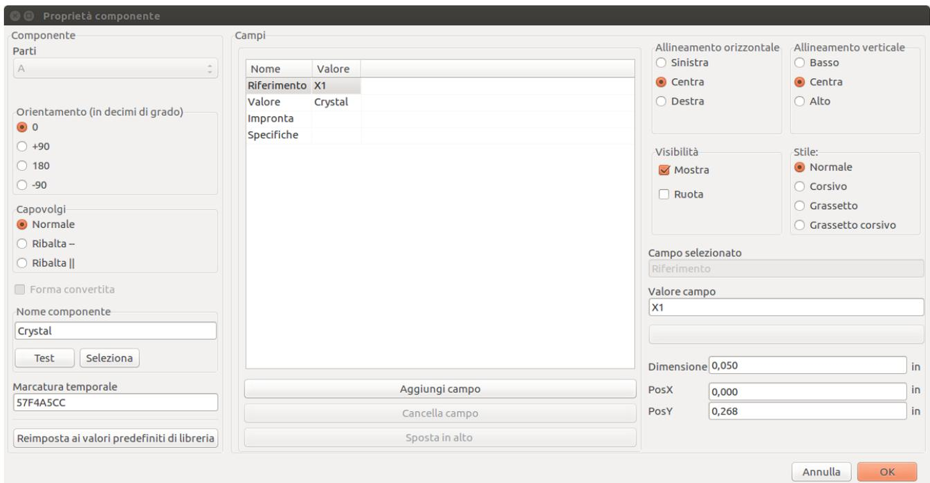
The Symbol Properties window displays all the fields of a symbol in a table. New fields can be added, and existing fields can be deleted, edited, reordered, moved, or resized. Fields can be arbitrarily named, but names beginning with `ki_`, e.g. `ki_description`, are reserved by KiCad and should not be used for user fields. All symbol fields will be added to the symbol's corresponding footprint when the [PCB is updated from the schematic](#).
