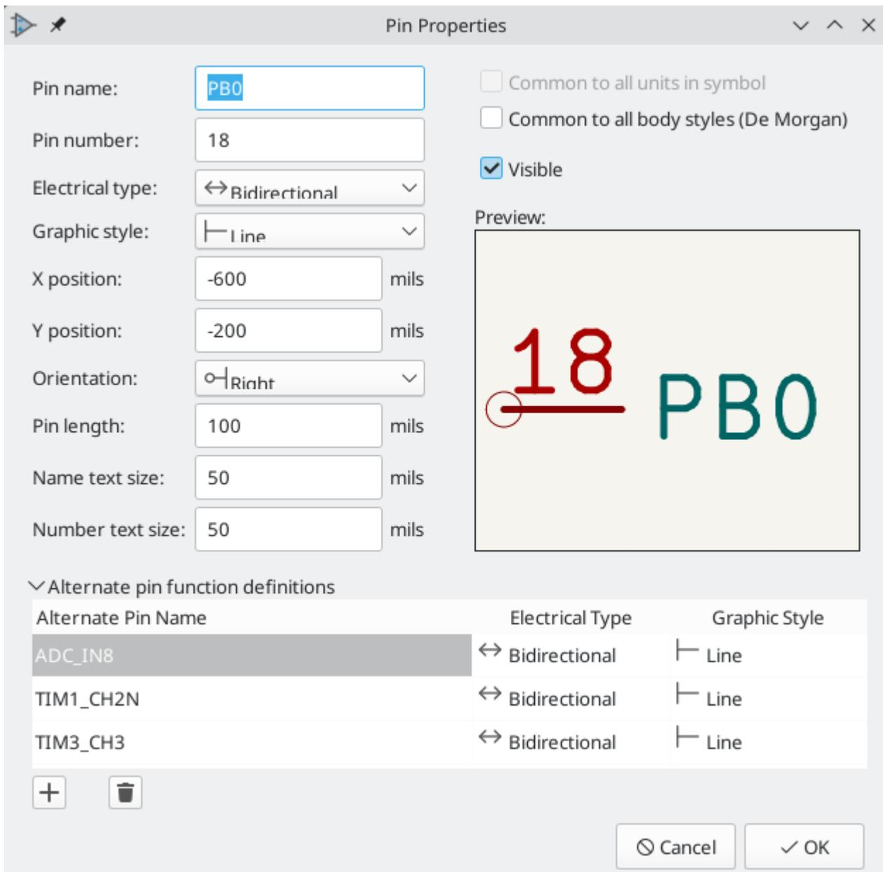
Alternate pin functions are selected in the Schematic Editor once the symbol has been placed in the schematic. For information on using alternate pin functions in the schematic, see the [schematic editor symbol documentation](#).
