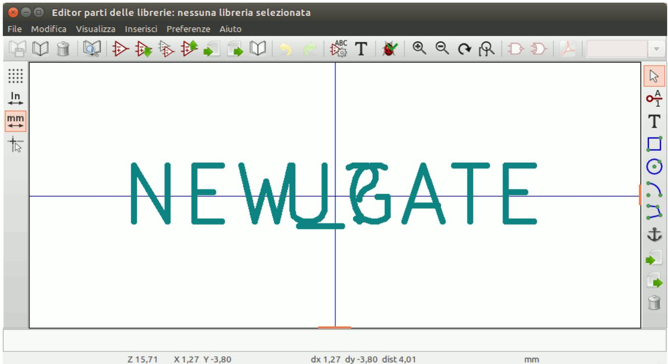
The blue cross in the center is the symbol anchor, which specifies the symbol origin i.e. the coordinates (0, 0). The anchor can be repositioned by selecting the
