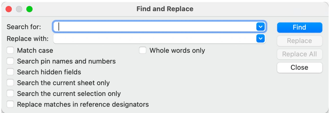
If the **Replace matches in reference designators** option is checked, reference designators will be modified if they contain matching text. Otherwise reference designators will not be affected.
