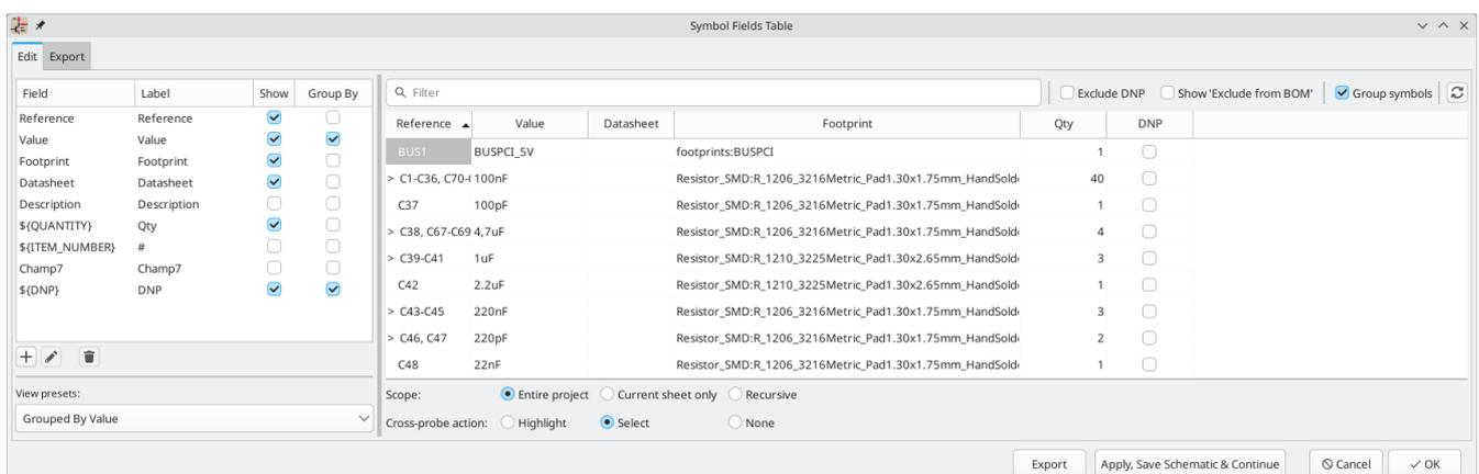
Fields with the **Show** box checked will be included as columns in the BOM, and fields with the **Group By** box checked are used to group components together. Components are grouped into the same line if all of their **Group By** fields are identical and the **Group symbols** box is checked. You can set an arbitrary column name for each field and reorder columns by dragging their headers.
