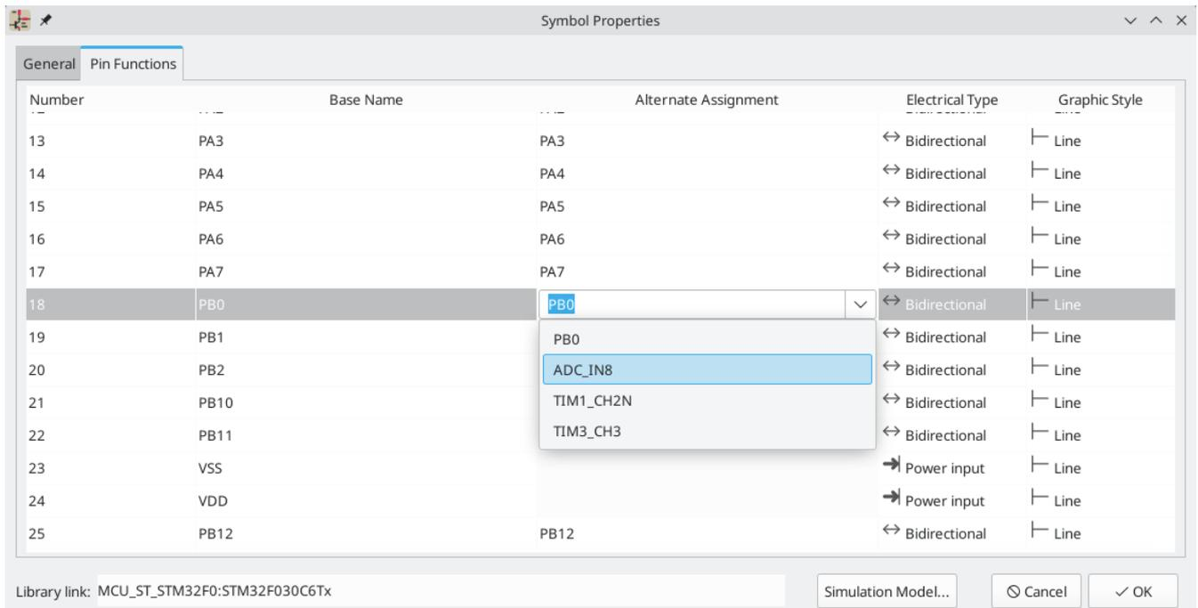
Pins that have alternate functions available are displayed with a small graphical indicator next to the pin name, as shown in the screenshot below. To globally show or hide these indicators, use **View** → **Show Pin Alternate Icons**.
