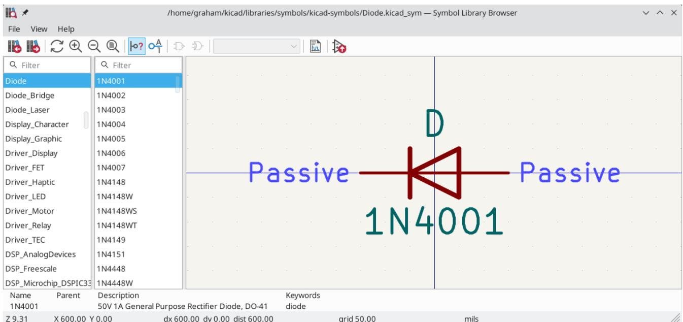
Double clicking the name of a symbol or using the
