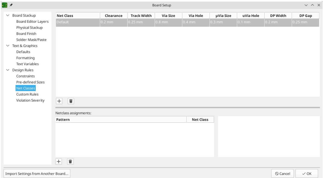
Track width and spacing can be managed manually by the designer during layout, but net classes are recommended because they provide an automatic way to manage and check design rules.
