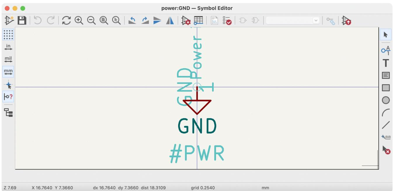
Power symbols consist of a pin of type "Power input" that is marked invisible. They must also have the **Define as power symbol** property checked. [Invisible power input pins](#) have a special property of making implicit global connections based on the pin name.
