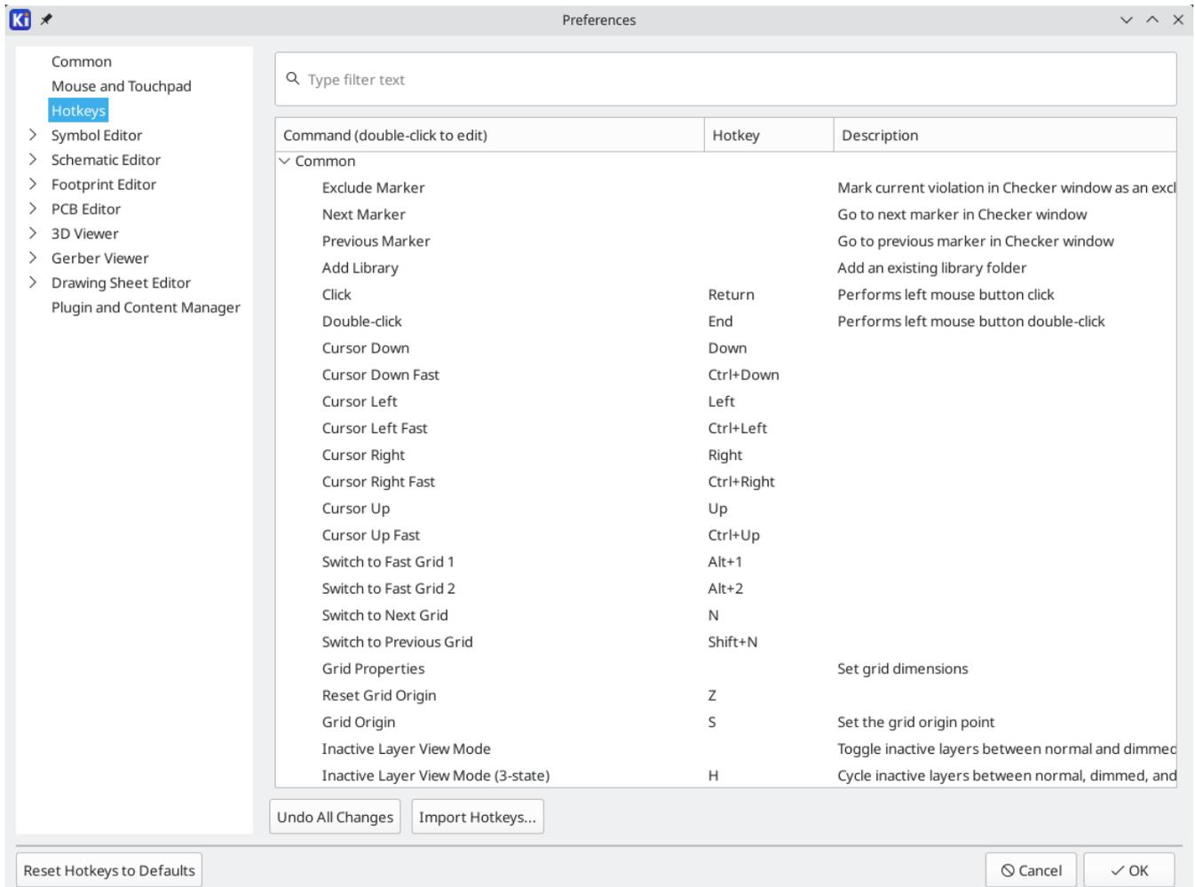
You can use this dialog to customize the hotkeys used to control KiCad. The hotkeys in the *Common* section are shared between every KiCad program. Hotkeys for each specific KiCad program are shown when that program is running. You can assign the same hotkey to a different action in different KiCad programs (for example, the schematic editor and the board editor), but you cannot assign a hotkey to more than one action in the same program.
