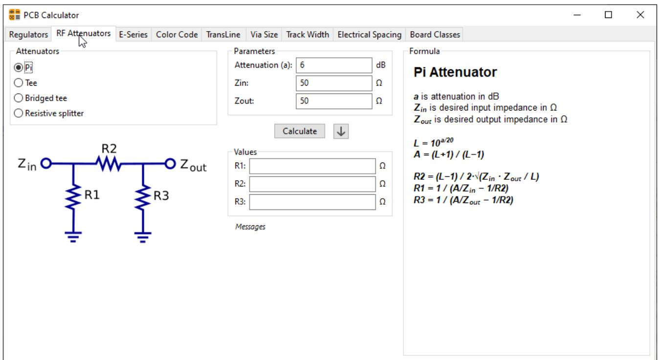
The screenshot shows the PCB Calculator software interface. The 'RF Attenuators' tab is active, and the 'Pi' attenuator type is selected. The parameters are set to: Attenuation (a) = 6 dB, Z<sub>in</sub> = 50 Ω, and Z<sub>out</sub> = 50 Ω. The circuit diagram shows a Pi network with resistors R1, R2, and R3. The formulas for calculating R1, R2, and R3 are displayed on the right.
