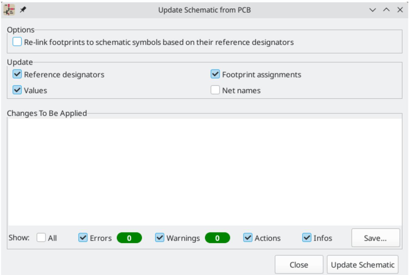
The tool syncs changes in reference designators, values, footprint assignments, and net names from the board to the schematic. Each type of change can be individually enabled or disabled.
