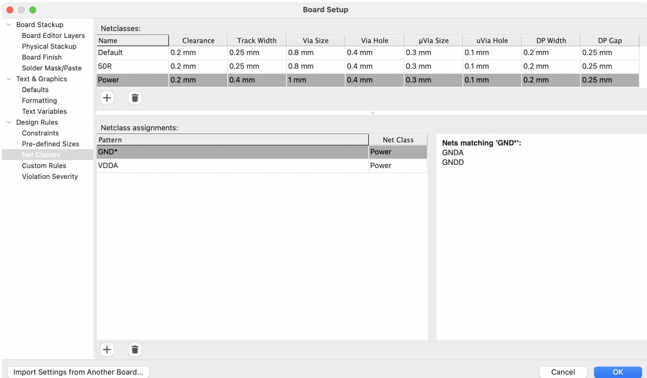
The upper portion of the Net Classes section contains a table showing the net classes in the design and the design rules that apply to each net class. Every class has values for copper clearance, track width, via sizes,
