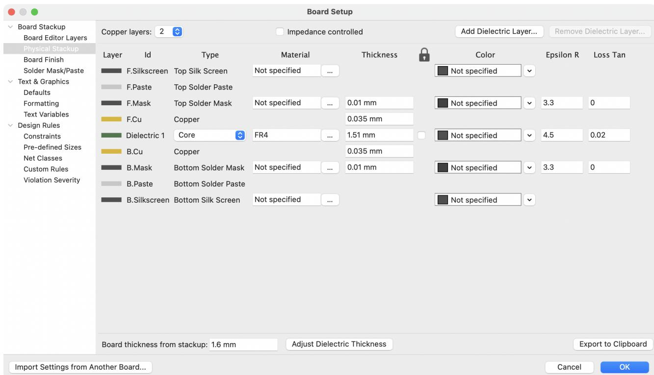
Set the number of copper layers in the upper left corner and then enter the physical parameters of the stackup if desired. These parameters may be left at their default values, but note that the board thickness value will be used when exporting a 3D model of the board. If you plan to use this feature, it is a good idea to ensure that the stackup thickness is correct.
