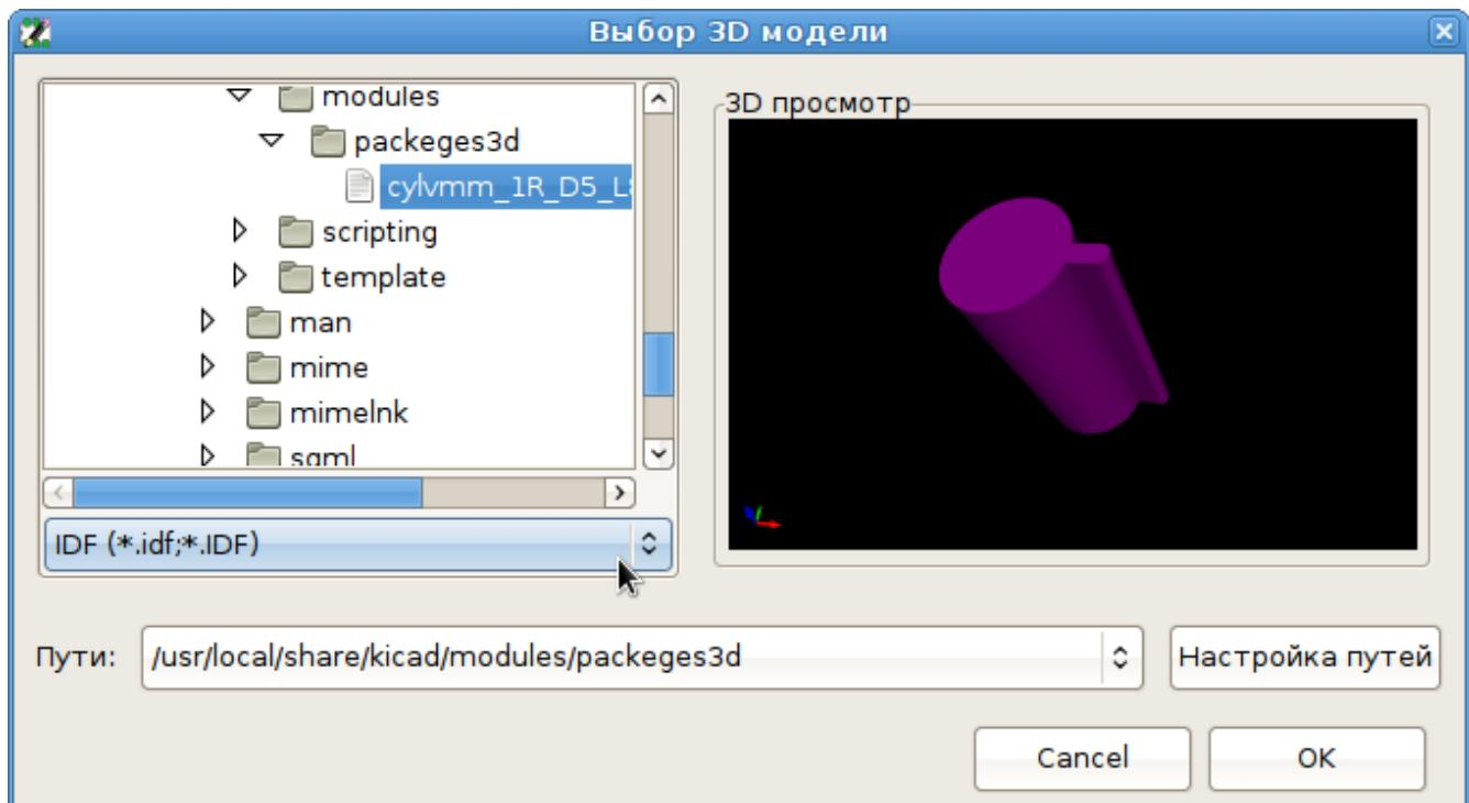
Once the desired component outline file is selected, enter any necessary values for the offset and rotation. The offsets must be specified using the IDF board output units (mm or mils) and in the IDF coordinate system, which is a right-hand coordinate system with +Z pointing towards the viewer, +X to the viewer's right, and +Y towards the upper edge of the screen. The rotation must be in degrees; positive rotation is a counter-clockwise rotation as described in the IDFv3 specification.
